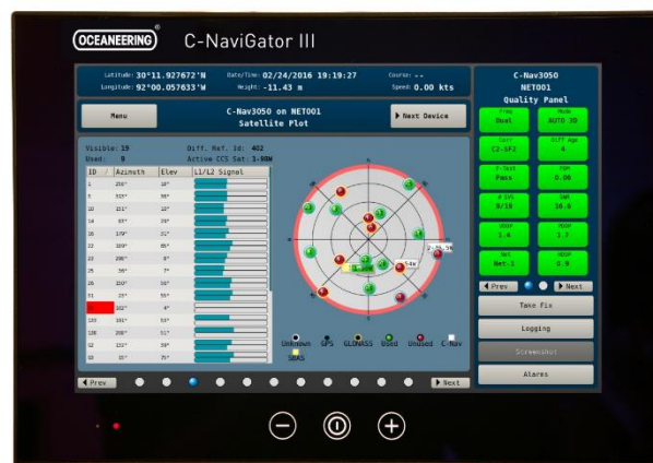
Figure 9: C-Nav Navigator III Control & Display Unit
